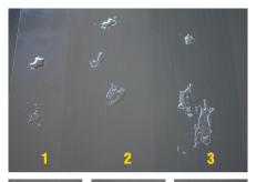
The picture shows a powder coated plate, where field 1 is untreated, field 2 is polished with 3D NanoProtect and field 3 is treated with MarineLakk.
