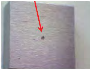
contact point (minimal wear)
