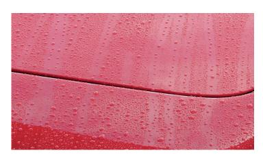
The treated surfaces show a very good drainage of water and a strong repellent effect on dirt.
